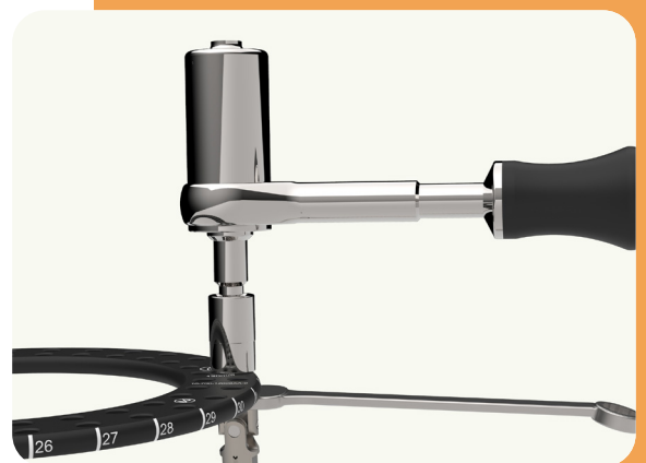
Fig. 16 - Tighten all Shoulder Bolt Connections
