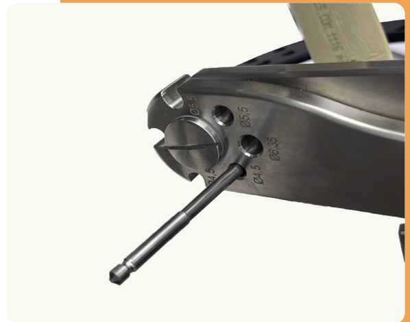
Fig. 20 - Trim Excess Wires/Pins
