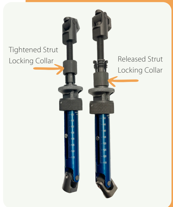
Fig. 17 - Tighten Strut Locking Collar
